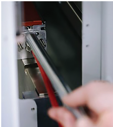
Quick seal die changes – most often in under 2 minutes – are one of CMD's fast-changeover design features.
