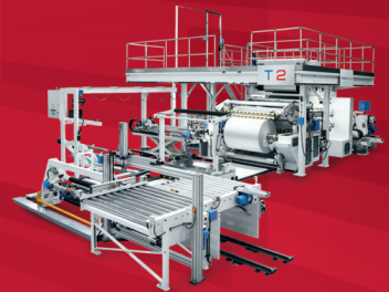
Slitter rewinders, pope winders, doctor machines for aseptic liquid packaging material
