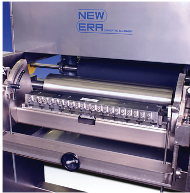
Photo 3 – Slot Die Coater
