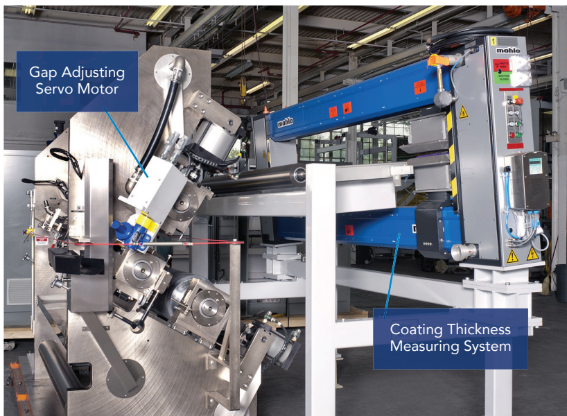
Photo 8 – Reverse Roll Coater with Closed Loop Speed and Gap Control
