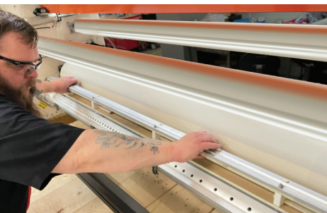
Enercon's new removable cartridge with quick disconnect electrodes.
