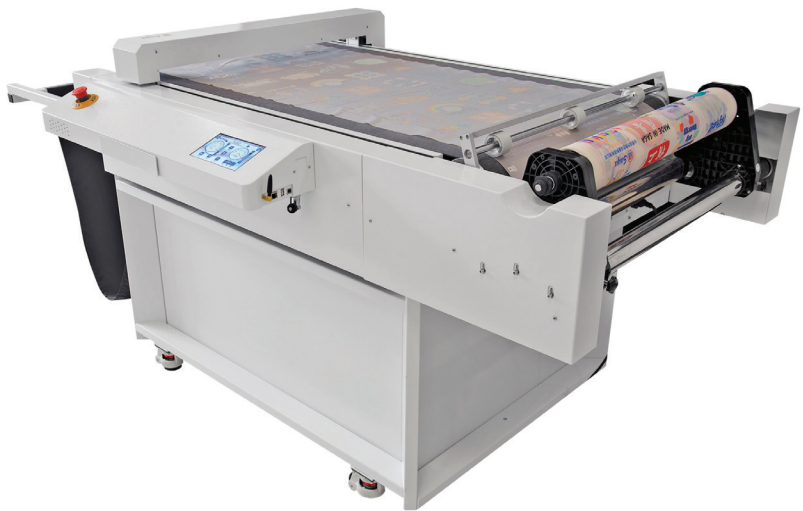
Digital die cutting utilizes computer-controlled machines to achieve unparalleled accuracy and flexibility. Photos courtesy of Supply55, Inc.
