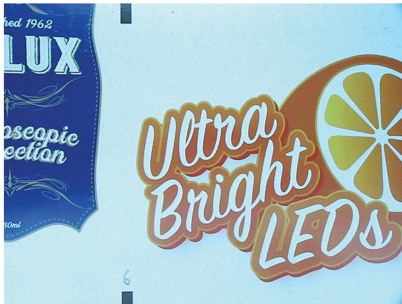
Figure 1: The print your eye sees on a final label. With macro inspection, an operator is able to see voids, skips, streaking, scumming (fogging), and out-of-registration defects.
