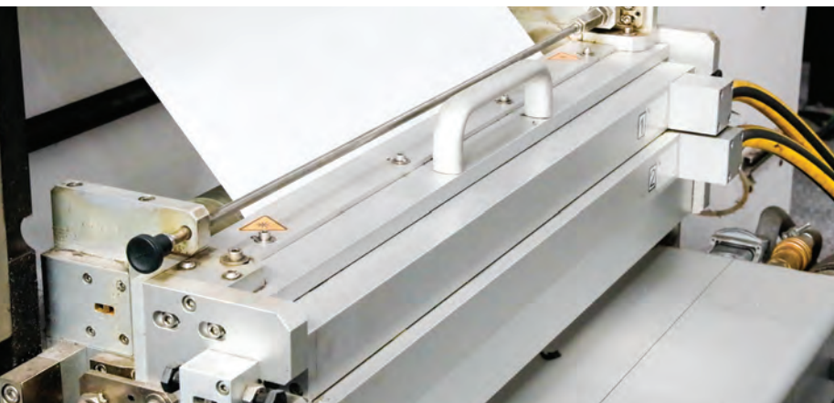
UV curing utilizes electricity instead of heat and provides an instant cure to silicone for less energy use and fewer harmful emissions.
