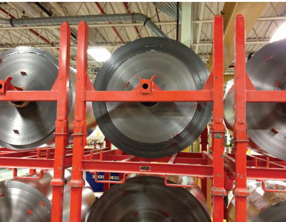
Using custom engineered storage and material handling racks can better protect high-profile wrapper products while requiring less space.
