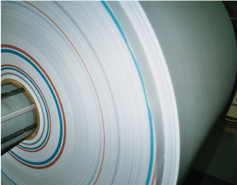
A roll which has been marked with an ink edge marking system. With edge markers, the entire defective section of a roll can be marked.
