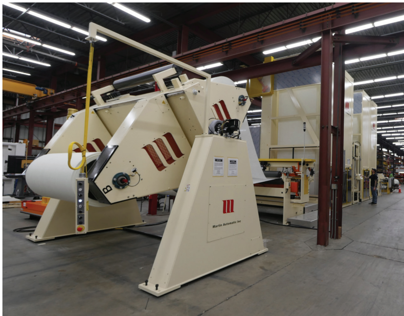
Designed to handle 2mm thick fiberglass for roofing shingles, the MTL takes 23 seconds to complete a splice on 1.7m wide web using hotmelt.
