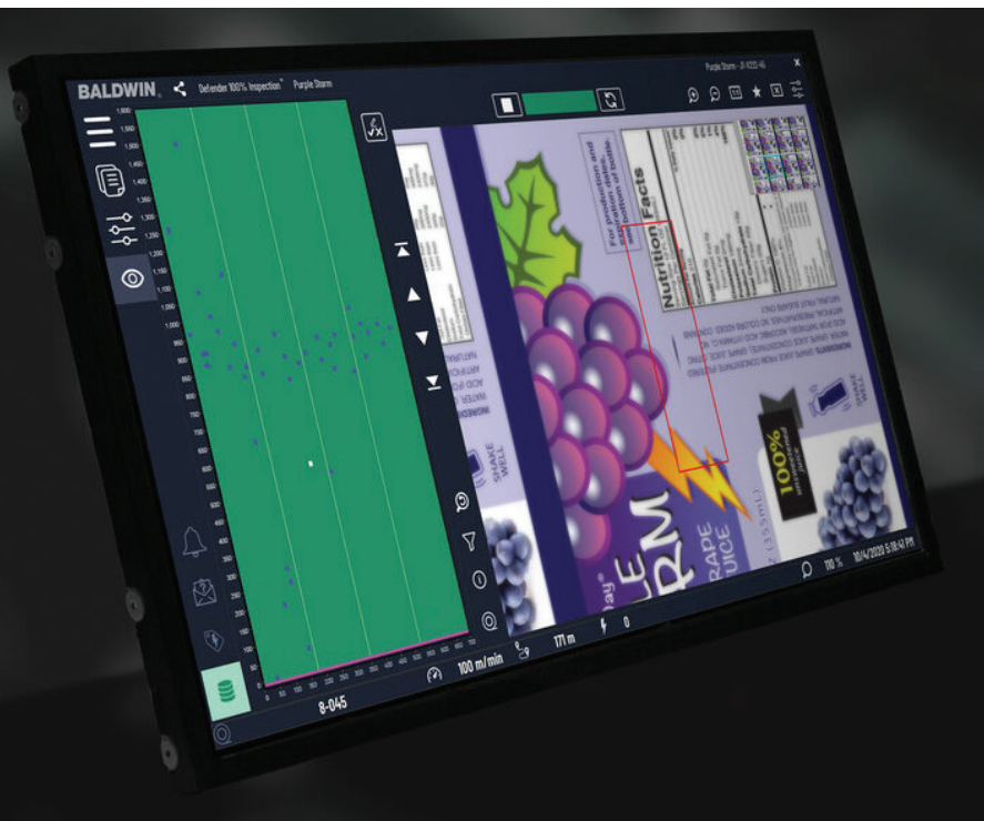
Equipment monitoring the entire web 100% of the time helps detect and manage defects.
