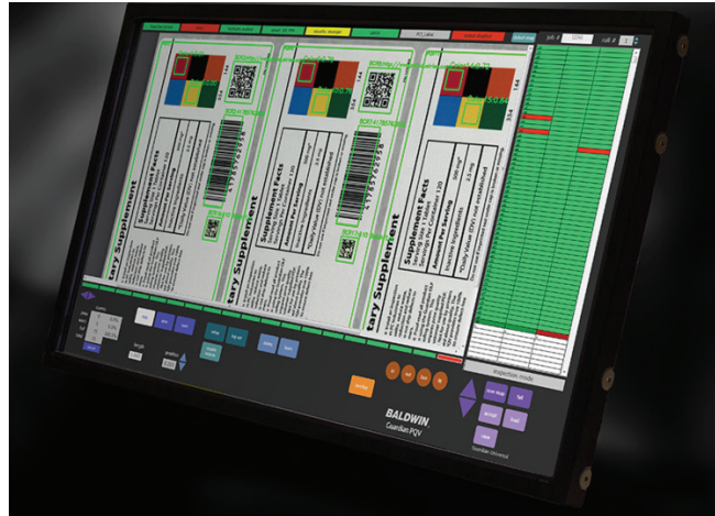
State-of-the-art camera systems can provide single or dual sided 100-percent print quality inspection for any application.
