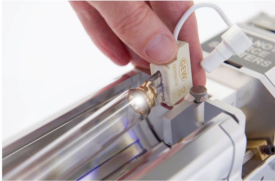
Figure 1: Between 10 and 100 mg of elemental mercury is contained inside conventional UV curing lamps. For reference, 5 mg of mercury covers the tip of a ballpoint pen.
